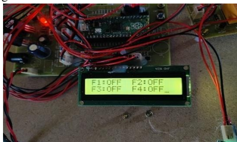
Figure 5: Fire sensors are OFF
